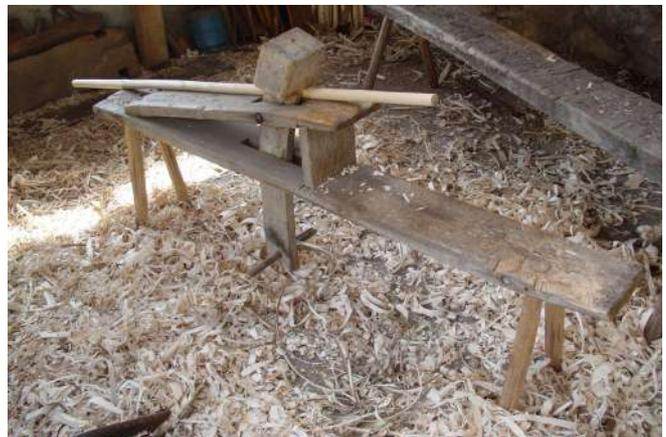
*A Shave Horse being used to produce a backsplat*
