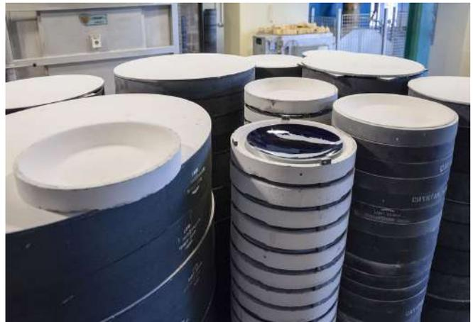
*Modern saggars at the Sevres Pottery Works these are probably made with alumina or silicon carbide ceramic*
